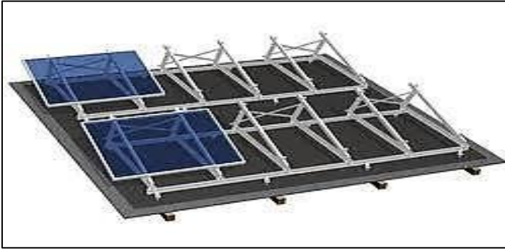
The Steel Structure on which the solar panels are fixed is the Solar Module Mounting Structure as shown in the picture.
